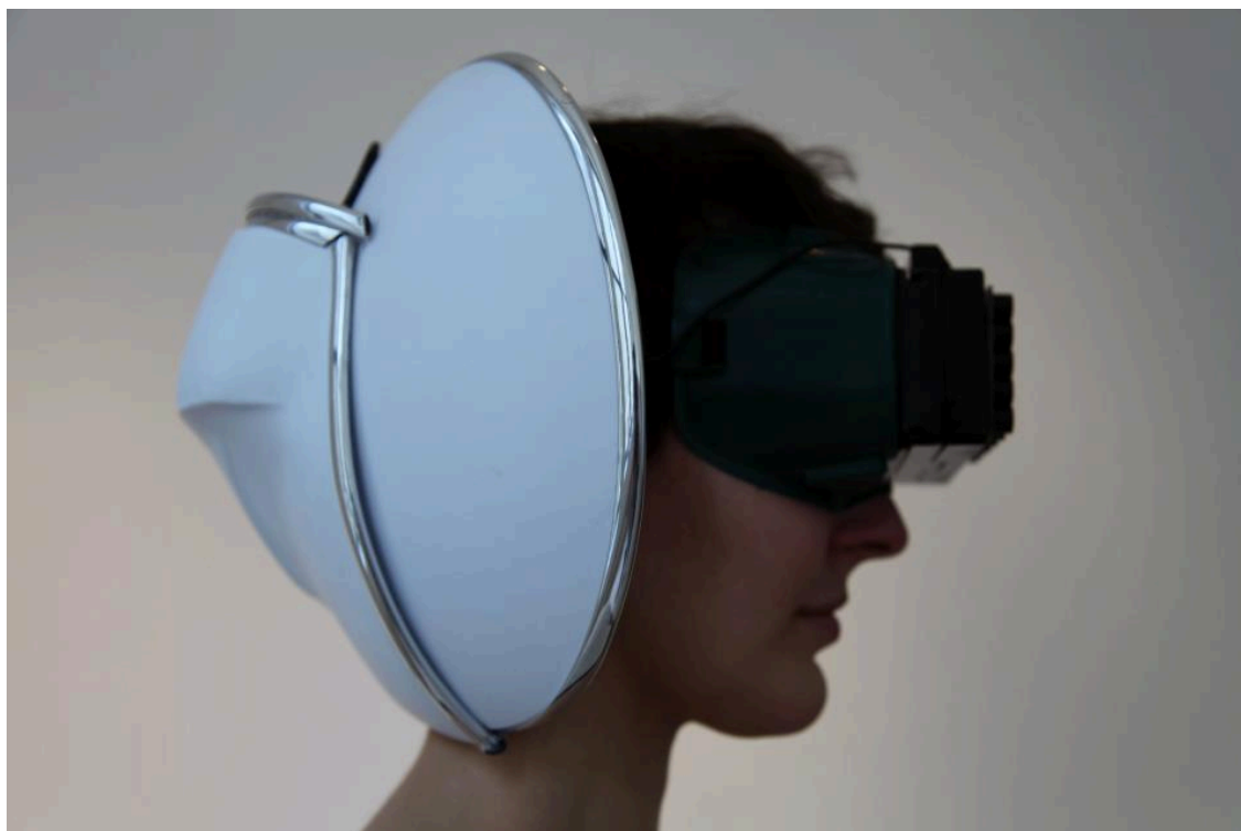
Fig. 3.29 Echolocation Headphones: Profile View
