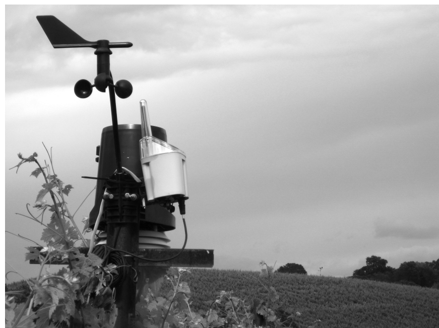
Fig. 2. Camalie Vineyard sensor station. Data is mapped to the physical modeling characteristics of a wave-guide physical modeling synthesis engine. The real-time output of the synthesizer is perturbed by the changes in the vineyard. (Photo © Mark Holler)
