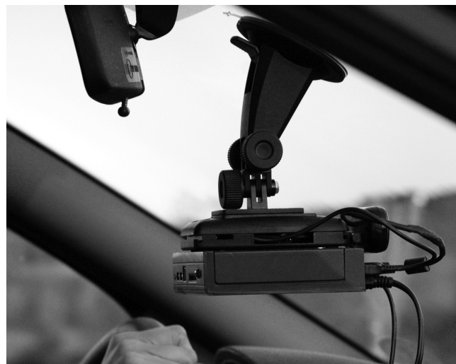
Fig. 1. RoadMusic device, 2012. RoadMusic is a live sonic experience in which music is created from the car ride itself. Accelerometers gather data about bumps, curves, accelerations and braking while a camera analyzes the visual scene through blob-tracking and color analysis. This data is used by custom software on a dedicated on-board computer to generate sound. (Photo © Peter Sinclair)
